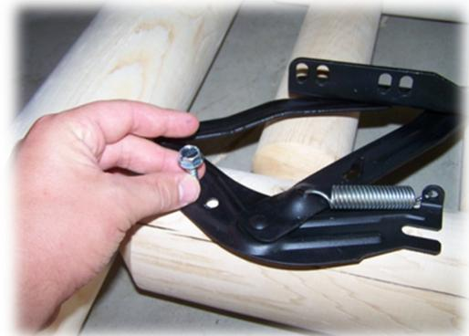
4. **Attach the back deck** first by lining up the holes in the deck to the holes in the hinge.
