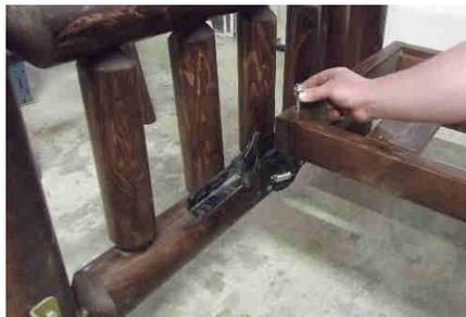
**7) Fasten Futon Deck Back** to Hinge using supplied  $3\frac{1}{2}$ " bolts as shown using  $\frac{1}{2}$ " wrench. Flat washer goes on top, bolt downward, nut on the bottom. Use outside slots on bracket that will result in decks being furthest apart.
