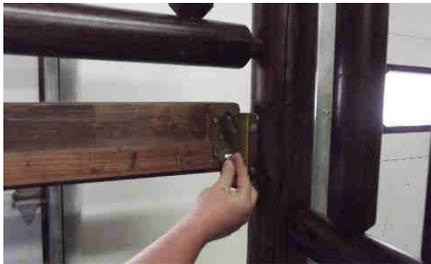
**4) Safety Rail, then Top Side Bed Rail:** Insert safety rail **first** (use mallet) **then**, install **Bed Rail**: Pre-fasten bolts one end, hook onto post bracket, screw-in bolts by hand on other end as shown.
