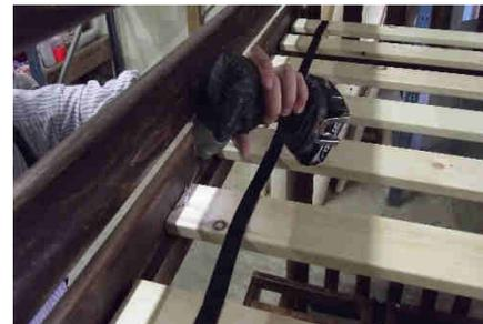
**9) Fasten Slat Roll to Bunk Bed Rails:** Stretch out Slat Roll and fasten through centre slat, then end slats to Bed Rails using wood screws (#2-Robertson) through pre-drilled holes.
