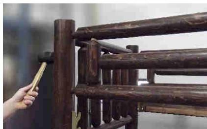
**5) Front Top Side-Rail:** Same as back side, Safety Rail first, then **Bed Rail**, screwing in bolts second end by hand as with back side. Tighten.
