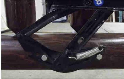
**2) Attach Bedrail Brackets** ( $5\frac{1}{2}$ " floor-to-bottom-of-bracket, pre-marked) Four per Bed End assembly (2 top, 2 bottom), Hooks go on the outside pointing up, Screws go on the inside.
