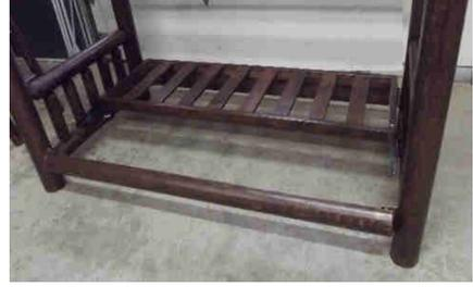
**6) Futon Deck - Back:** Position onto hinge as shown (back has no gripper pad like the Deck Front)
