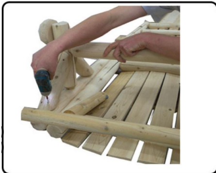
3) Insert Log Brace on one side, then on other side. (wheels out). Insert 4 screws – 2 on each side.
